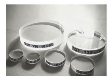
Optical flats are mainly used for the measurement of the surface flatness of polished surface for checking the flatness using monochromatic light source. The main applications of optical flats are listed below:
