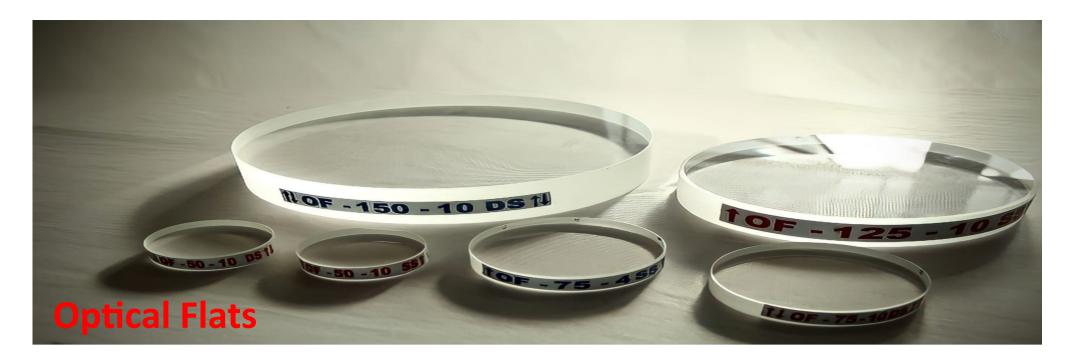
Optical flats are mainly used for the measurement of the surface flatness of polished surface for checking the flatness using monochromatic light source.
